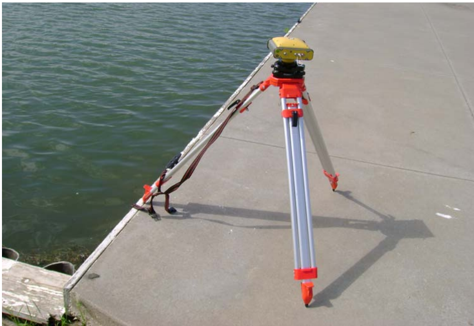
Figure 3b. Close-up view. Lake level was measured from the water surface to the top of the concrete pad at the eastern edge (left in picture) of the concrete.
