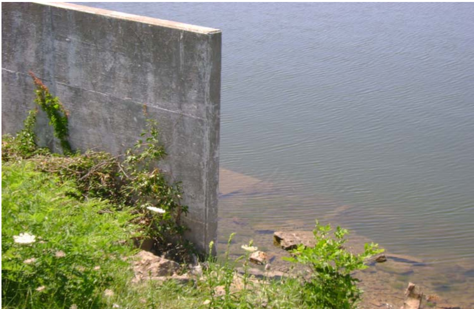
Figure 3b. Close-up view. Lake level was measured from the water surface to the top of the concrete wall at the eastern (right side in picture) side.
