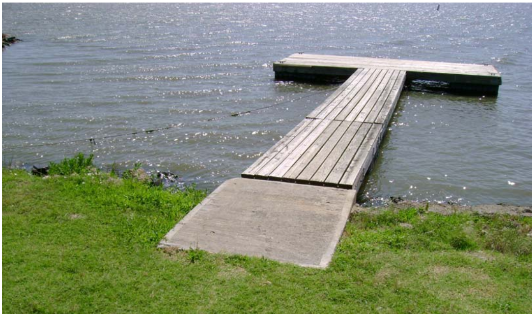
Figure 3b. Close-up view. Lake level was measured from the water surface to the top of the concrete pad at the southern edge (left in picture) of the concrete.
