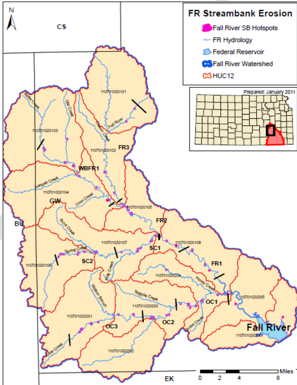
Figure 6: Upper Fall River Watershed Streambank Erosion Assessment by Stream Reach & 12-digit Hydrologic Unit Codes (HUC12)
