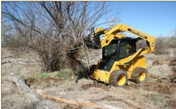
"JAWZ" ATTACHED TO A JOHN DEERE 250 SKIDSTEER MACHINE EXTRACTING A TAMARISK PLANT, WITH ROOT.
